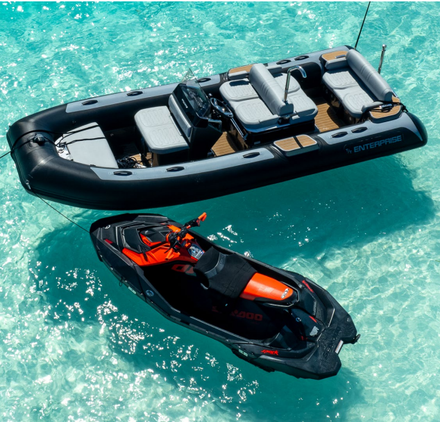
5m (16.6ft) Williams 505 tender with inboard diesel jet engine
